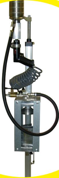
AutoDrain's Unique water and sediment separation system is included as standard with your Fuel Tank Drill. This ensures that you retrieve clean, reusable fuel from End of Life Vehicles. This separation system also serves a dual purpose as a sight glass. Both single and double options are available depending on your business needs.
