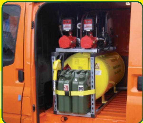
The Mobile Fuel Scavenger can be fitted for side or rear door access, allowing you to fit an RDT to the rear of your van if needed. This allows you to create a dual-purpose vehicle, saving both time and money.
