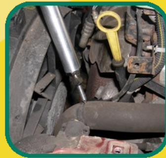
Coolant spike piercing the hose
