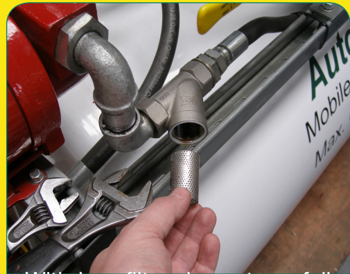
Withdraw filter element carefully and remove any debris. Refitting is the reverse of removal.
