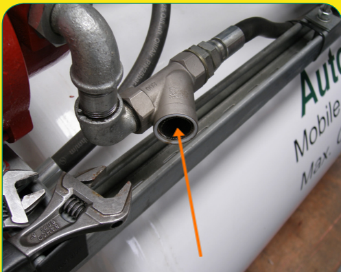
Unscrew filter element retaining cap from filter housing
