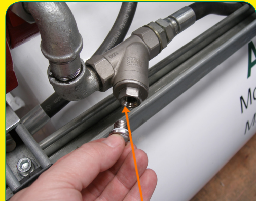
Remove drain plug first to allow any excess fuel to drain away
